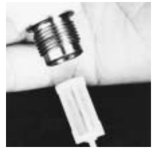
A DISPOSABLE NYLON MESH FILTER FITS NEATLY INTO THE NECK OF THE PAINT CUP.
